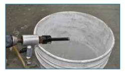
**Step 1** Attach the water swivel (central water feed) and wet core diamond bit to the drill. Connect the water swivel to a water source and adjust the water flow to a slow trickle. Constant, slow water flow will reducing chipping by cooling and lubricating the drill bit.
