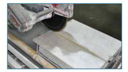
**Step 1** Cover the saw tray with a piece of ¼" cement board. This will provide a continuous surface that supports the sheet during cutting and prevents mosaic pieces from falling into the tray's cutting channel.
